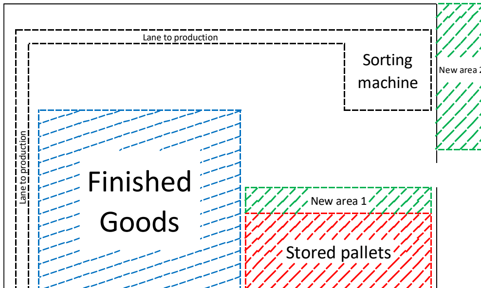
Figure 20: New structure of the pallet warehouse.
