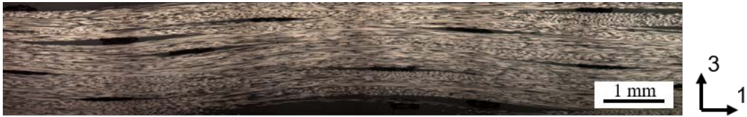
Figure 1: Micrograph of a section in test specimen B2-1, which reveals the fibre waviness out-of-plane. The black regions are weft yarns in the NCF.
