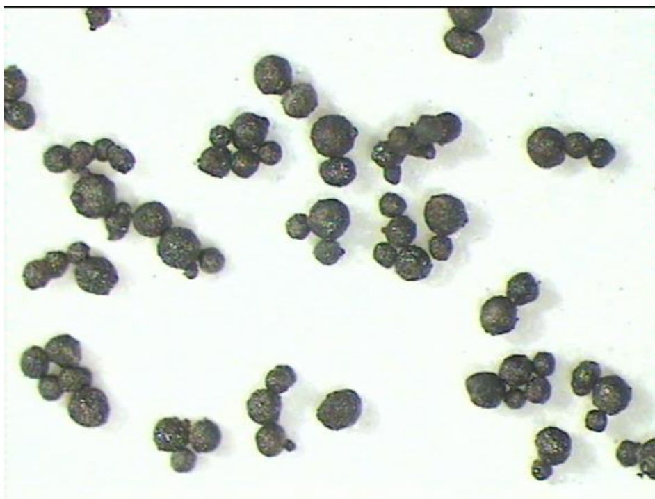
Figure 3.4.3 Light microscope image of unused spray dried particles. Small satellites are attached to some of the larger particles.
