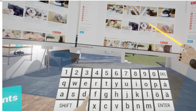
Figure 5.17: The system keyboard. The user can press a key by enabling the poke action on the controller and touching a key.
