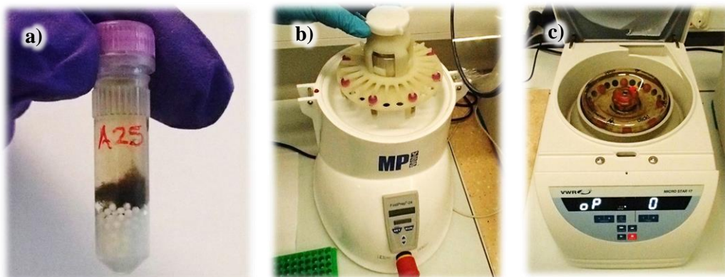
Figure 11: a) Prepared sample solution in LME tube prior to homogenisation; b) FastPrep®-24 homogeniser; and c) VWR Micro Star 17 centrifuge.
