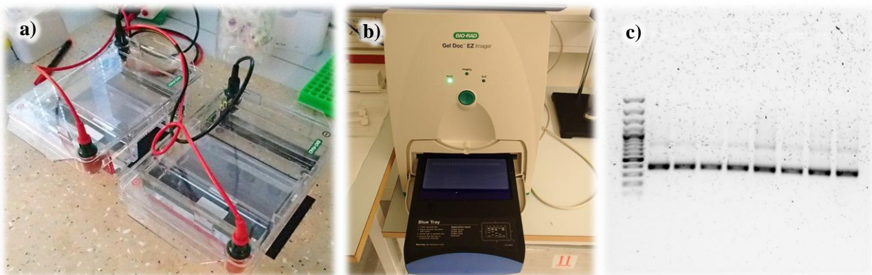
Figure 15: a) Gel electrophoresis chambers; b) Gel Doc™ EZ Imager; and c) Example of a gel electrophoresis image produced using the Gel Doc™ EZ Imager and Image Lab™ software.
