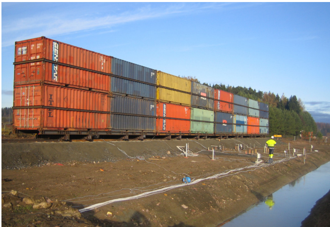
Figure 3.2: Perniö test embankment with the placement of loading carts and measuring instrumentation before the test procedure ( Lehtonen et al., 2015 )
