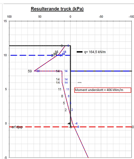
Figure E.2 Calculated lateral earth pressure during the design of the Tennet 2 project (Edmark & Hansson, 2011a).
