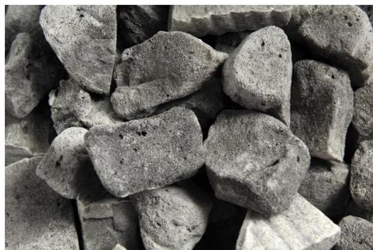
Figure 3.30: GEOCELL® foam glass gravel [100].
