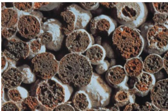
Figure 3.29: Cross-section photo of Lightweight Expanded Clay Aggregate [101].
