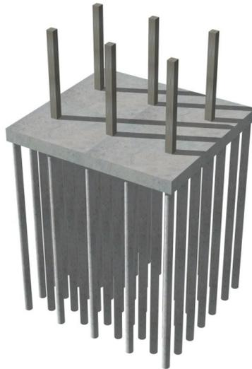
Figure 3.17: Typical arrangement of piles and columns in piled raft solution.
