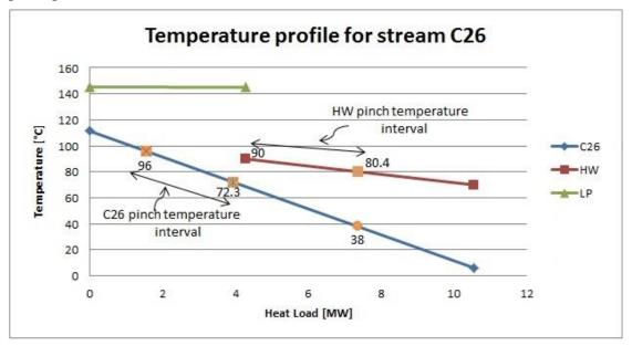
Figure 23.Temperature profile for heating of drying air in the bark dryer. The heating is done by firstly preheating the air with HW and then heating with LP steam. In the figure the pinch temperature intervals for both the drying air (C26) and the HW are shown.
