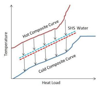
Figure 21. Hot and cold composite curves including an illustration of heat exchanging with the secondary heating system water.
