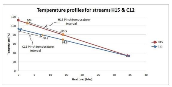
Figure 22. Temperature profiles for streams H15 and C12. In the figure the pinch temperature intervals for the hot and cold streams are shown.
