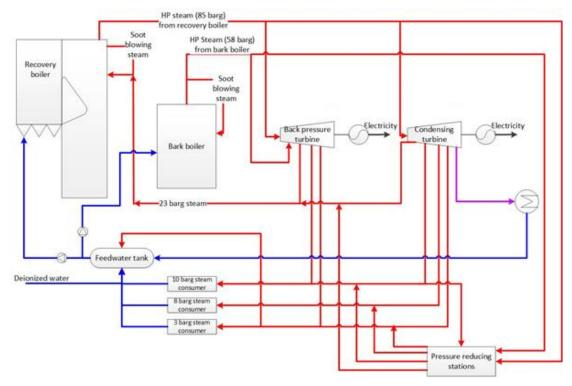
Figure 5. Steam network at the mill including for instance the two turbines and the different steam pressure levels required in the process (Rudén, 2017).
