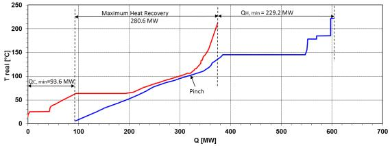
Figure 12. Hot and cold composite curves of Värö mill.
