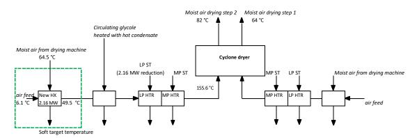
Figure 16. New moist air-air heat exchanger for the cyclone dryer. The HX is placed before the circulating glycol, LP and MP heating. The result is a 2.2 MW decreased demand for LP steam.
