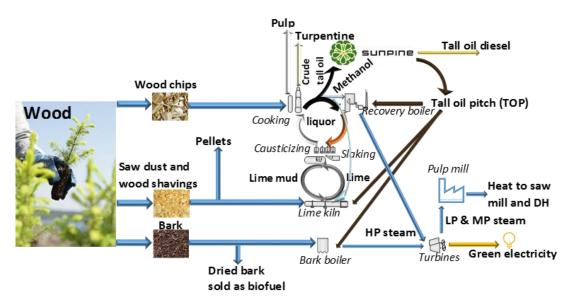
Figure 1. Energy and material flows at Södra Cell Värö site (Rudén, 2017).
