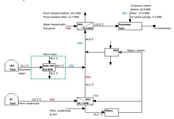
Figure 14. Retrofit proposal for the RB flue gas cooling and feed water heating. The dashed green lines show where the new heat exchanger is suggested to be installed. The resulting LP steam saved is 5.5 MW.
