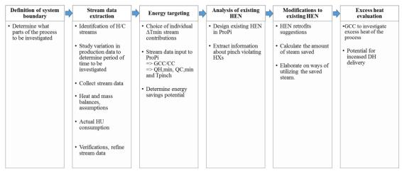
Figure 11. Procedure for the data extraction and energy analysis performed during the thesis.
