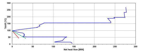
Figure 20. Background/foreground analysis for the delivery of DH to Varberg. The blue curve represents the GCC curve for the process with a global  $\Delta$ Tmin of 21 K (background). The red line represents the demand for DH during the investigated time period and the green dashed line represent the total delivery that the process in theory can manage.
