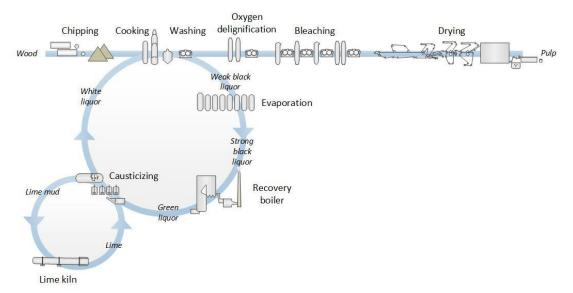
Figure 4. Simplified layout of the Kraft process showing some of the most important process steps (Rudén, 2017).
