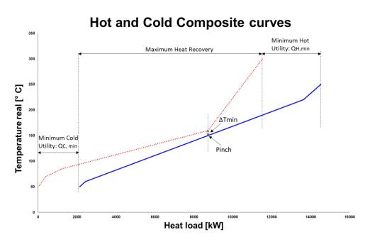
Figure 9. An example of hot and cold composite curves plotted in the same T/Q diagram. The dotted line, i.e. the above red curve, represents the hot composite curve. The filled line, i.e. the lower blue curve, represents the cold composite curve.
