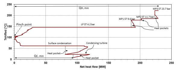
Figure 13. The GCC of Värö mill.
