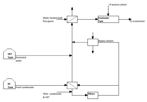
Figure 6. The condensate system at Värö.
