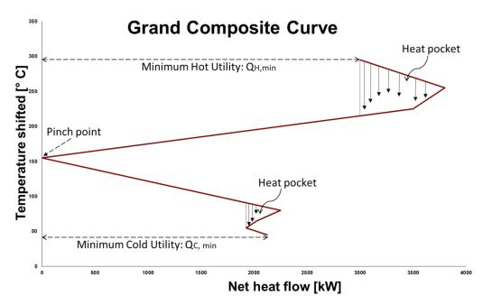
Figure 10. Grand composite curve example indicating some of the information that can be obtained for such a plot.
