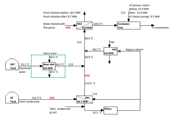
Figure 18. Further mitigation of the pinch violation related to the recovery boiler flue gases heating boiler feed water. Here, with utilization of the existing HW heat exchanger and in addition retaining the suggested new WW heat exchanger. A total of 9.5 MW LP steam is saved in the feed water tank.
