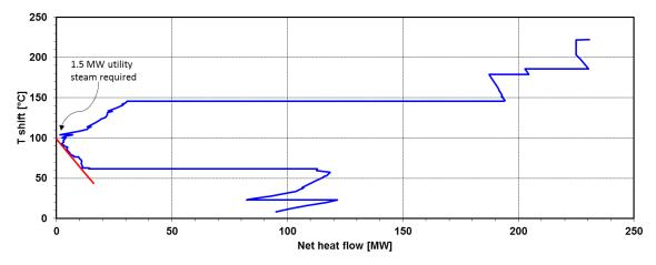
Figure 19. Background/foreground analysis of district heating delivery to Varberg. The blue curve represents the GCC of Värö mill (background), while the red line represents the demand for DH during the investigated time period (foreground). The black arrow in the figure depicts where the process excess heat does not match the DH demand. 1.5 MW LP steam would be sufficient to reach the DH target temperature and thus the demand.
