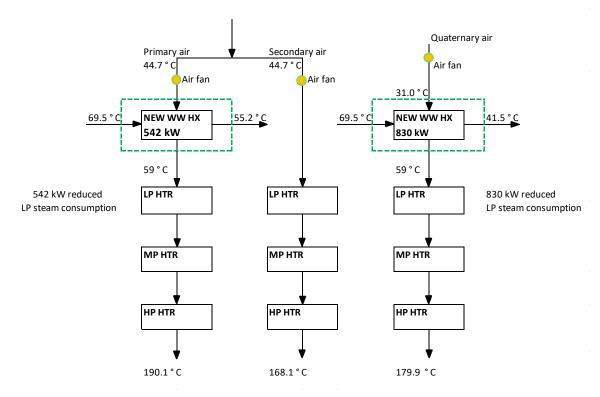
Figure 15. Retrofit proposal for combustion air to the recovery boiler. The two new heat exchangers use WW to preheat the primary and quaternary combustion air intakes enabling a steam savings of 1.4 MW.
