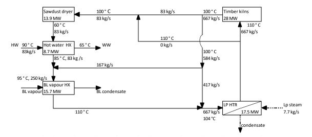
*Figure 8. How heat is provided to the pressurized circulating water for the sawdust dryer and the timber kilns.*
