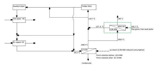
Figure 17. Introduction of a flue gas cooler to heat hot water to the saw mill. The flue gases arise from combustion of bark in the bark boiler. With this retrofit, 2.1 MW LP steam is saved.
