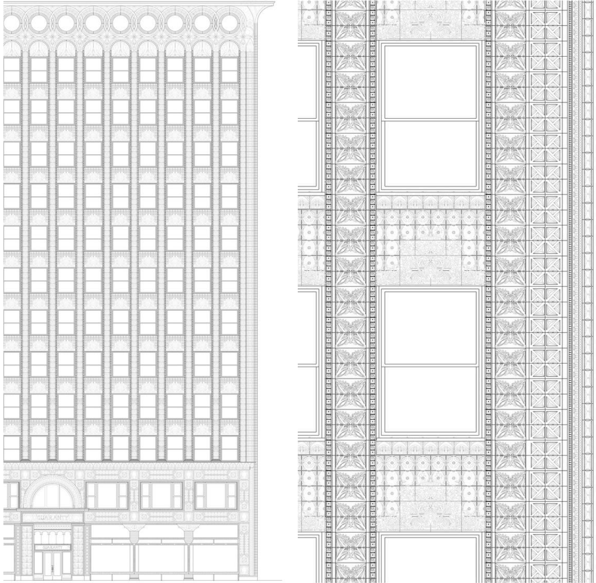
FIGURE 11 Sullivan's Guaranty Building. The building is very complete and harmonious as one form, yet the intricacy is continuing down the scales to each terra cotta tile. Drawings from Caruso ETH Studio
