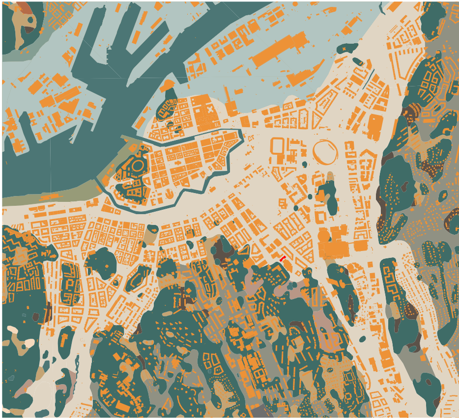
FIGURE 20 The soil composition of Gothenburg, it's Geology, have shaped the city. Own map based on data from Lantmäteriet (2017). The project site has quite favourable conditions with bedrock just 6-9 meters below the post glacial clay.
