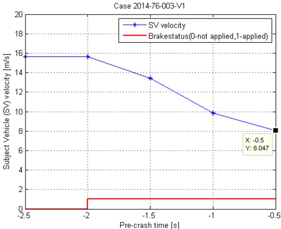
Figure 4.2: Raw data showing SV velocity, pre-crash time-series and brake status
