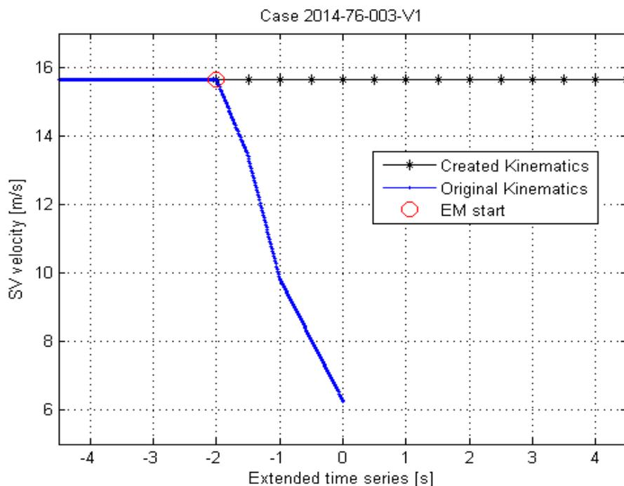
Figure 4.5: Creation of artificial kinematics for What-if simulations
