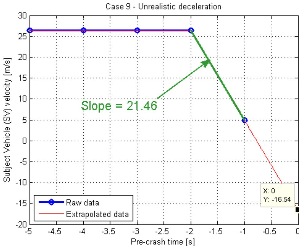
Figure 6.1: Velocity-time curve showing overestimated deceleration of Case 9
