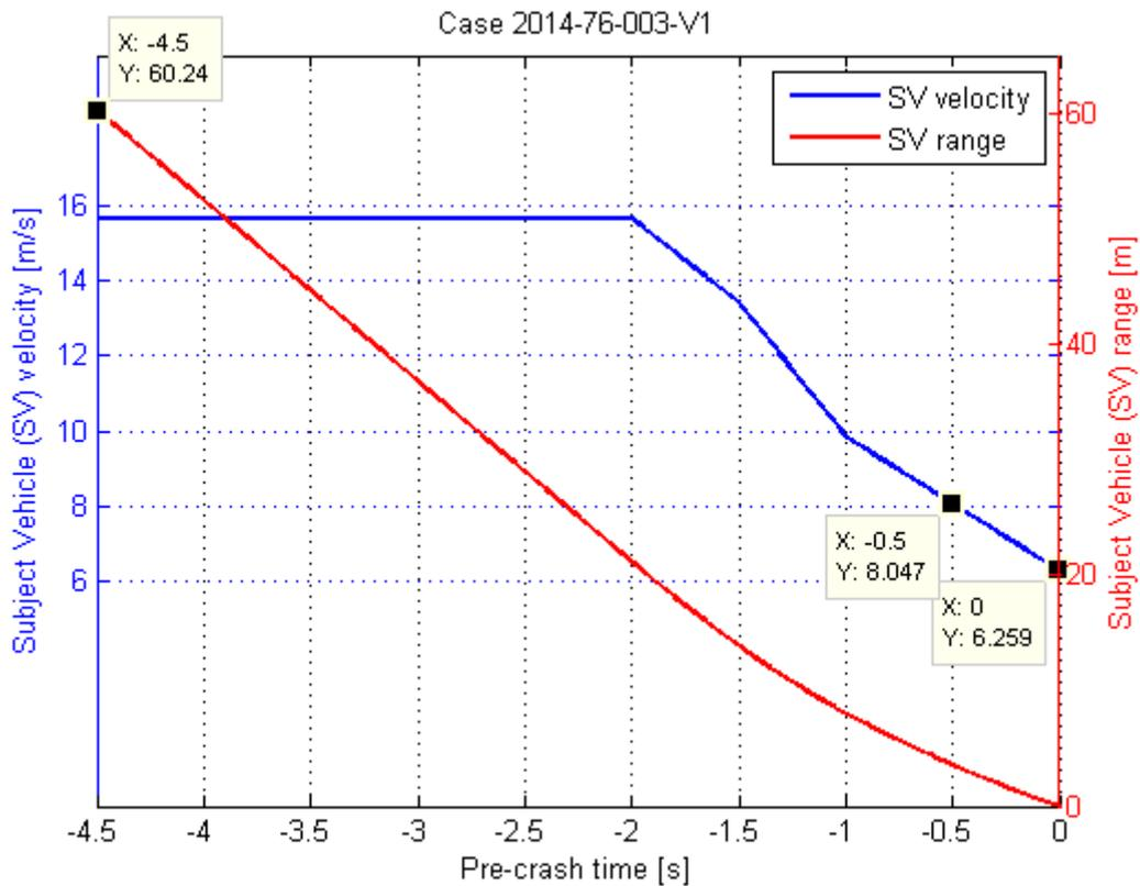
Figure 4.3: Effect of extrapolation on Impact speed (blue) and calculated distance (red).
