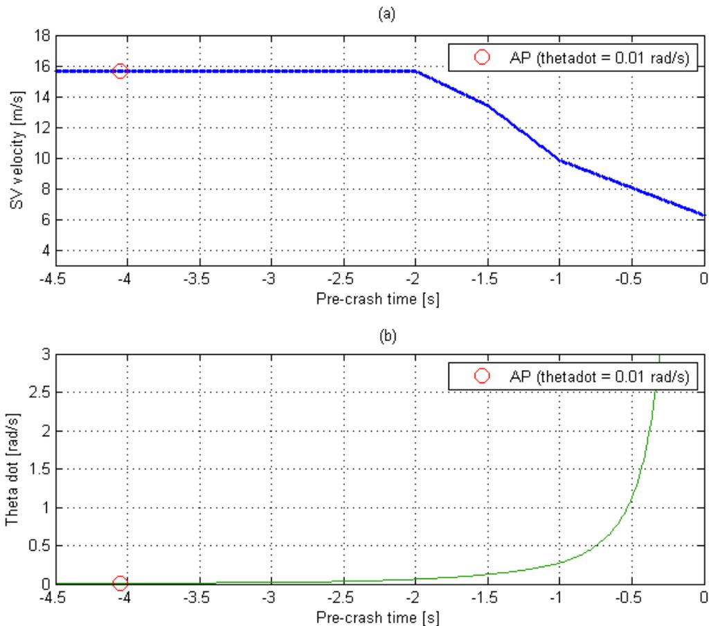
Figure 4.6: (a) Anchor point as seen from SV's perspective, (b) Variation of thetadot w.r.t SV kinematics
