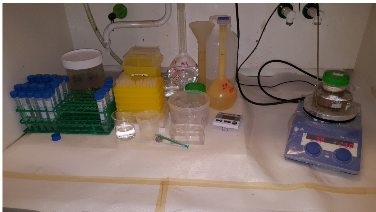
Figure 4. Experimental set up for the leaching process of molybdenum
