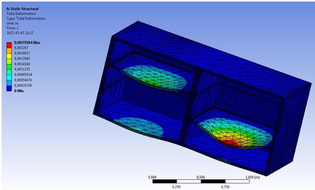
Figure A.20: Total Deformation for the minibox with shelves
