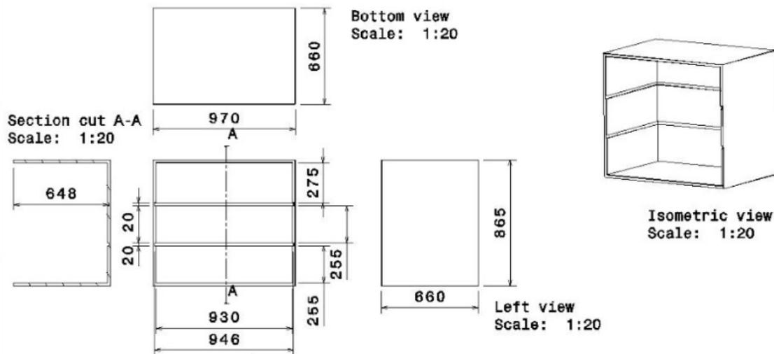
**Figure 11.7:** Technical drawing of the further developed storage space in the back with submersible function, small box inside the shell.
