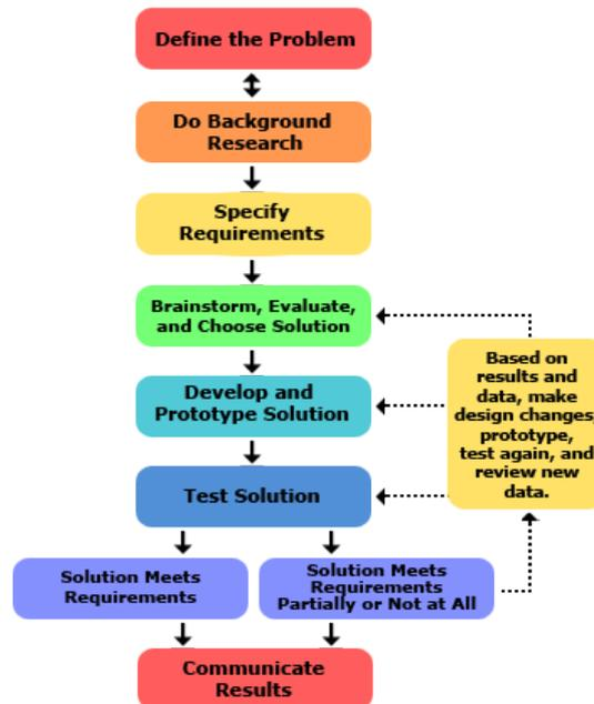
**Figure 3.1:** The engineering design process [1]
