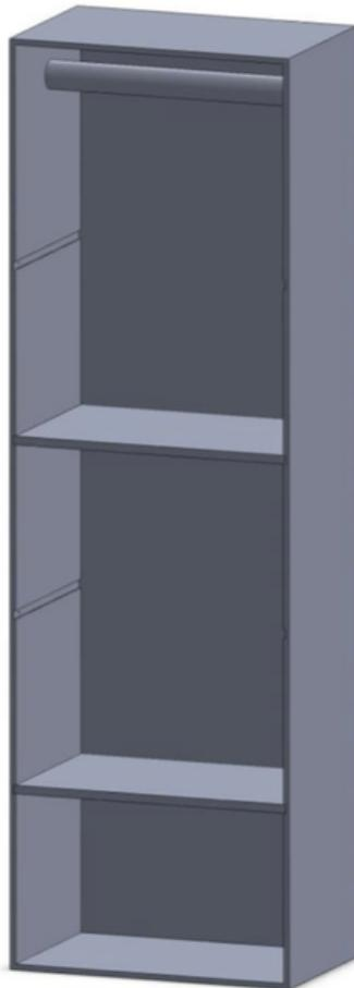
**Figure 8.1:** Isometric 3D CAD model of storage space located behind the driver and passenger seats.
