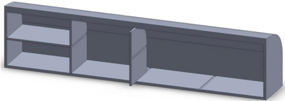
**Figure 8.2:** 3D CAD model of the front upper storage space.
