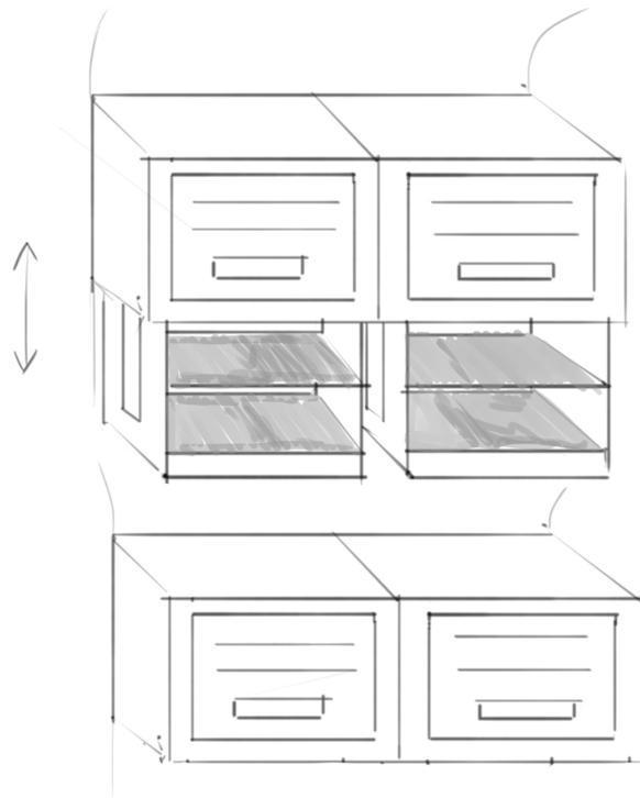
**Figure 11.1:** Rear storage with submersible function.
