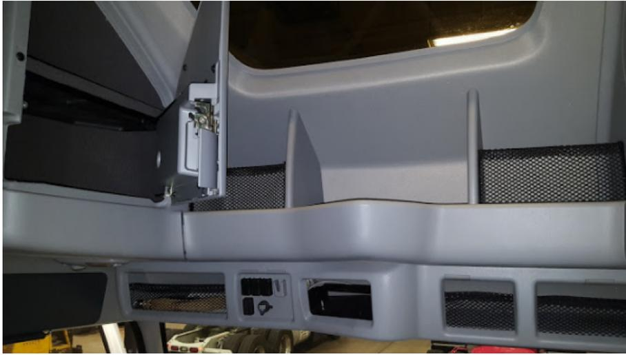
**Figure 4.4:** Current storage solution behind the driver for the European model. [2]
