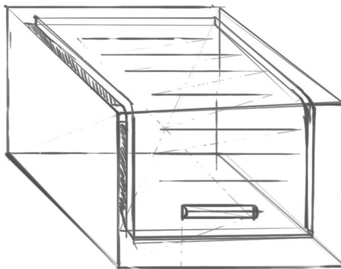
**Figure 7.11:** The Vertical sliding door.
