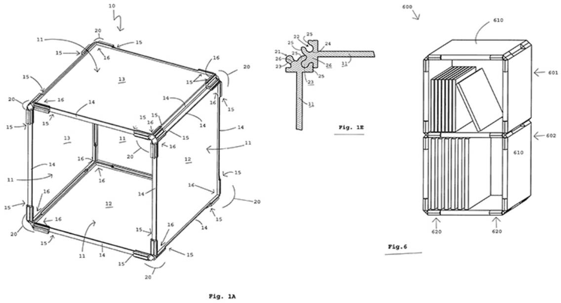
Figure A.14: Modular Storage in Passenger Compartments. [9]
