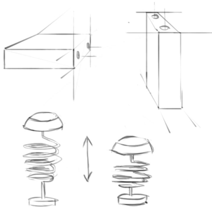
**Figure 7.14:** Spring-loaded pin.
