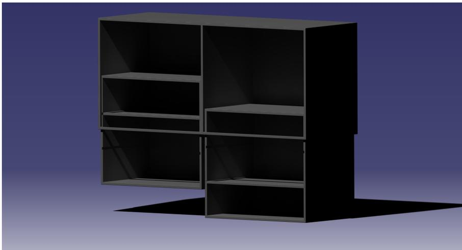
**Figure 11.6:** CAD-model of rear storage with submersible function.
