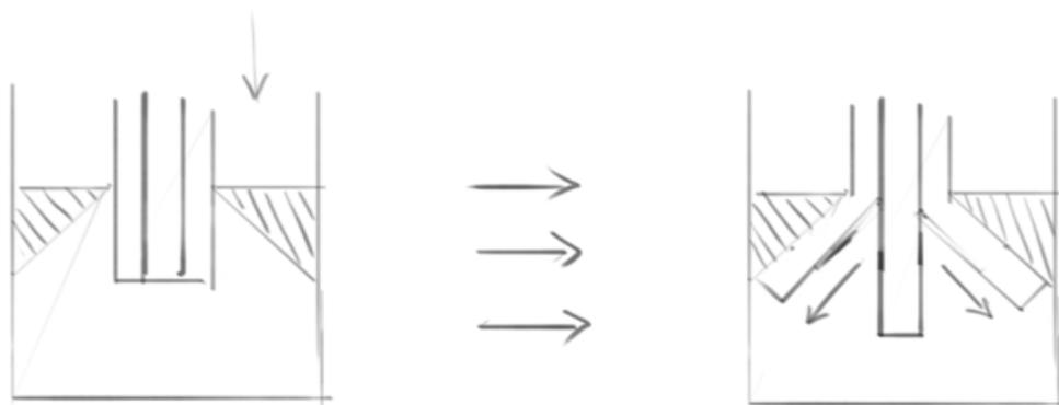
**Figure 7.15:** Fan locking mechanism.
