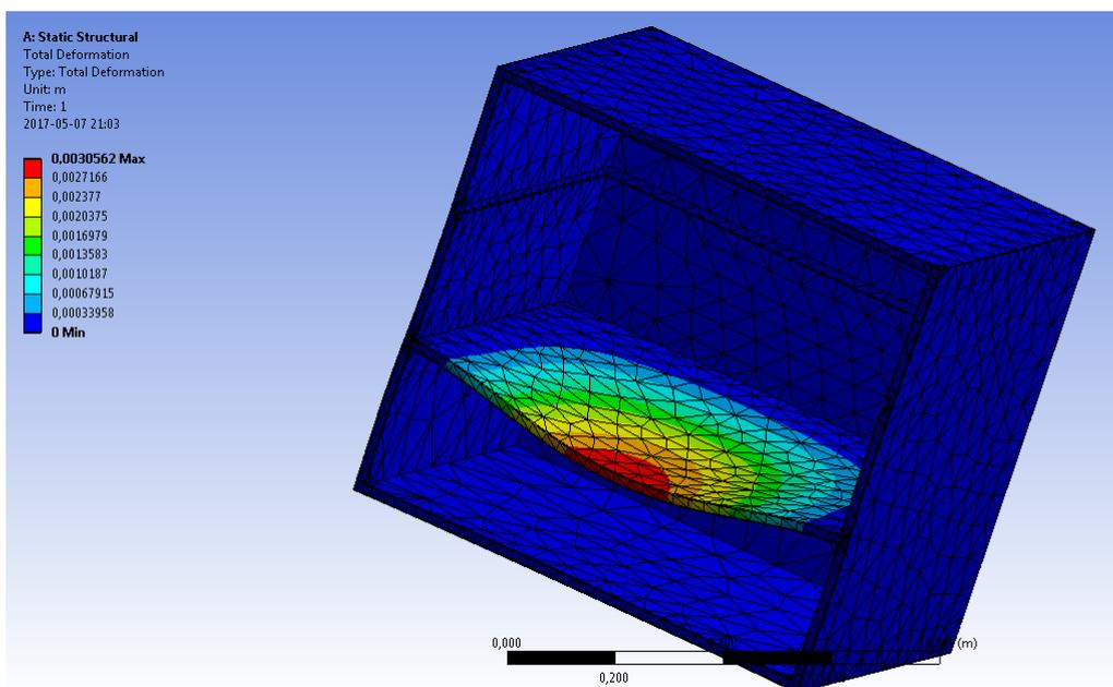
Figure A.19: Total Deformation for the minibox with shelves
