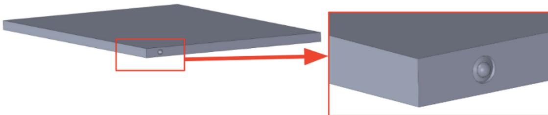
**Figure 8.6:** 3D CAD close-up of shelf with spring-loaded ball pins.
