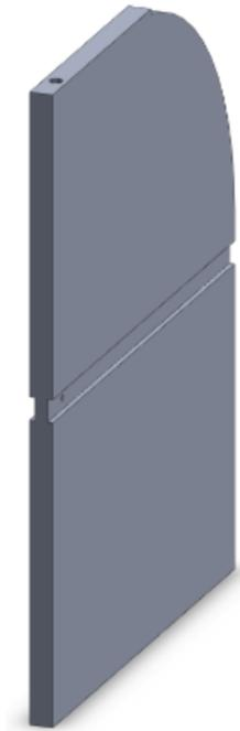
**Figure 8.5:** 3D CAD close-up of the vertical divider with slotted tracks.
