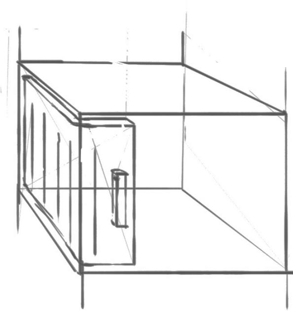
**Figure 7.10:** The Horizontal sliding door.
