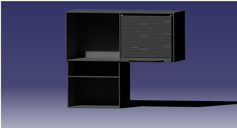
Figure A.15: CAD-model of rear storage with submersible function.
