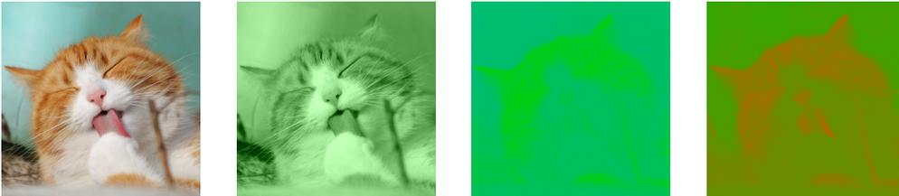
**Figure 2.3:** The different channels of the color space YCbCr. From the left: full image, the luma channel (Y) and the two chroma channels (Cb) and (Cr) in that order. In the luma channel edges are abstracted from the color compositions. Best viewed in color.
