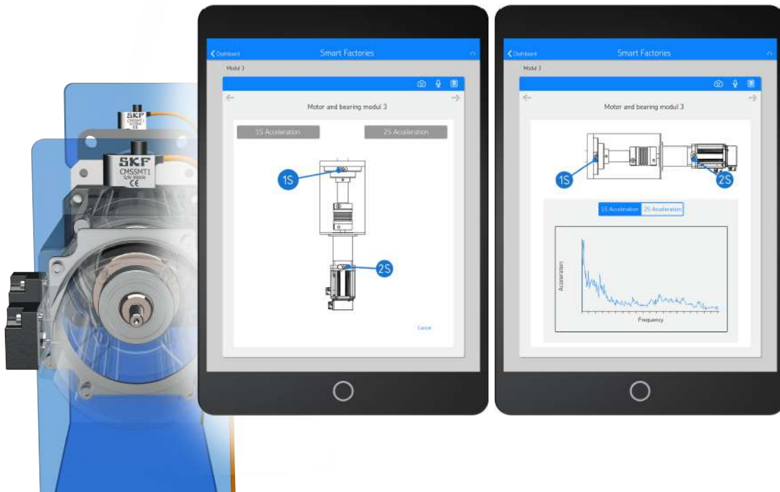
Figure 4.7: Illustration of SKF-Enlight connected to the vibration sensors
