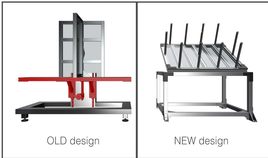
Figure 4.1: Comparison between the old and new design of the Storage table, movable parts that have been removed completely.
