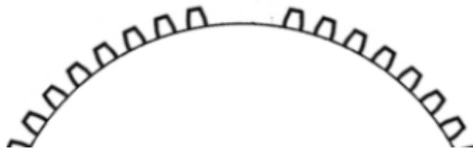
**Figure 2.1:** *Illustration of the detection points on the flywheel. The gaps (missing teeth) of detection points that are used to establish absolute position are also illustrated. The engine considered in this project have three of these gaps, separated by 18 teeth.*
