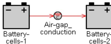
**Figure 3.8:** Modelling heat transfer between battery cells.
