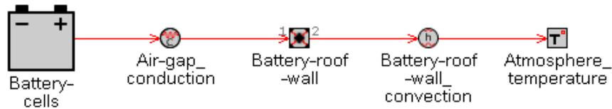
**Figure 3.7:** Modelling heat transfer from battery cells to the surrounding air outside the module.
