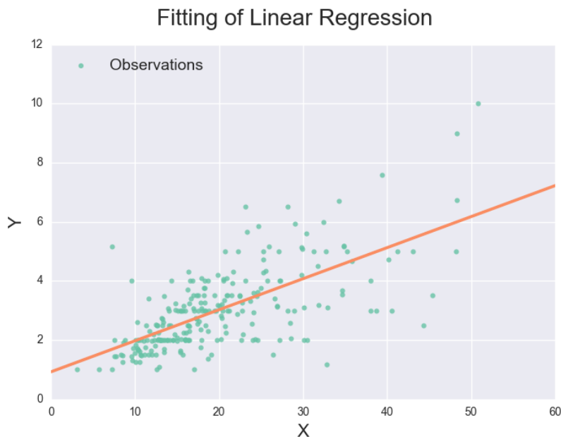
Figure 2.1: The principle of linear regression visualized
