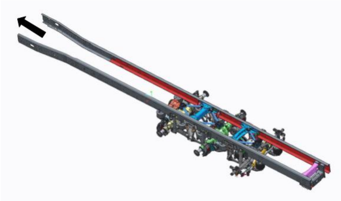
Figure 4.2-1. CAD template assembly (only rear axles mounted on the chassis frame, the arrow indicates the travel direction of the vehicle).
