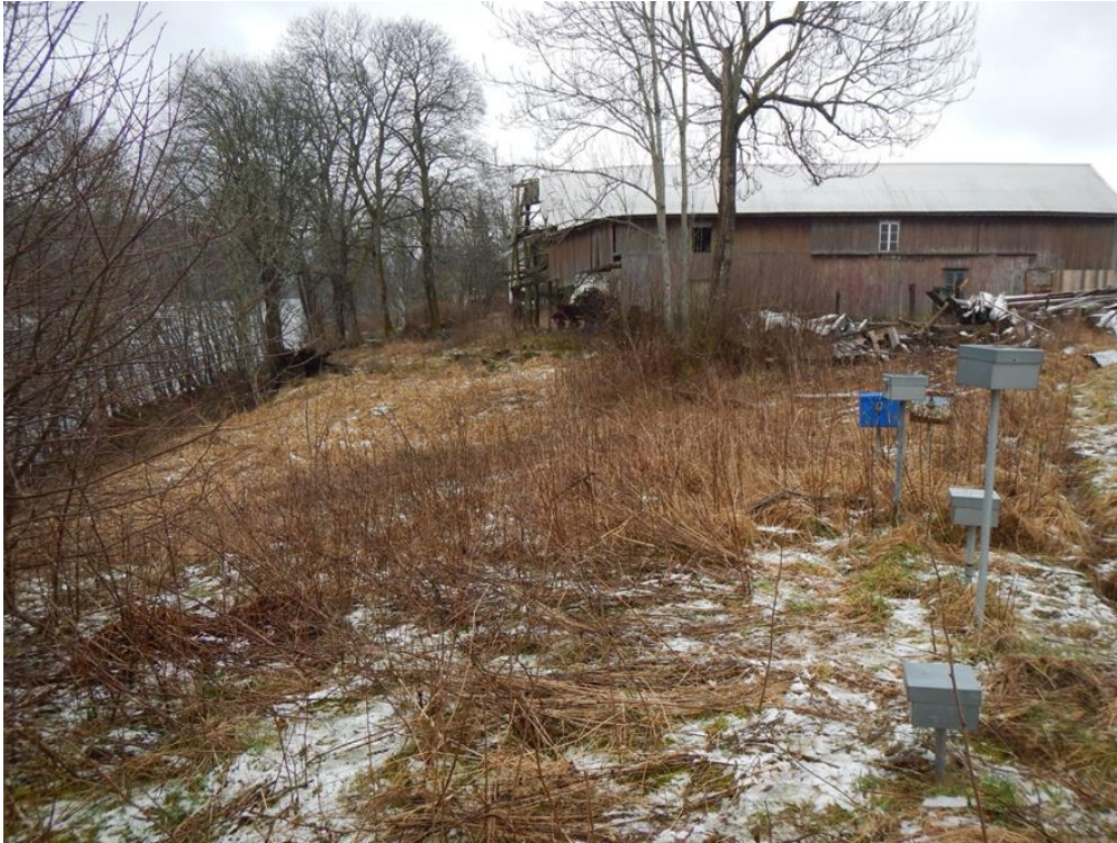
Figure 4-12. Piezometers at the crest of the slope, picture taken towards south. An old cowshed in the back.
