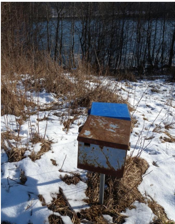
Figure 4-10. Piezometers at the toe of the slope. As can be seen the station is placed some meters from the shore due to the vegetation and the coarse erosion protection material placed next to the river.
