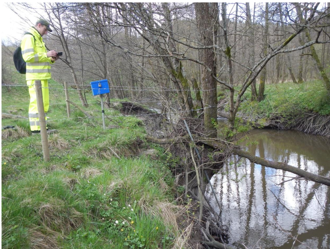
Figure 5-47. Piezometer installed in Lärje River, the blue box contains the logger.
