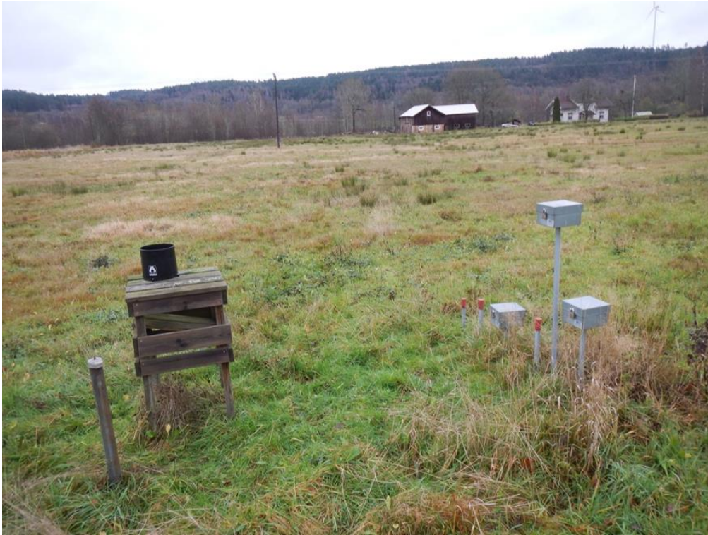
Figure 4-14. Piezometers and the precipitation gauge at the back of the slope. Picture taken towards east.
