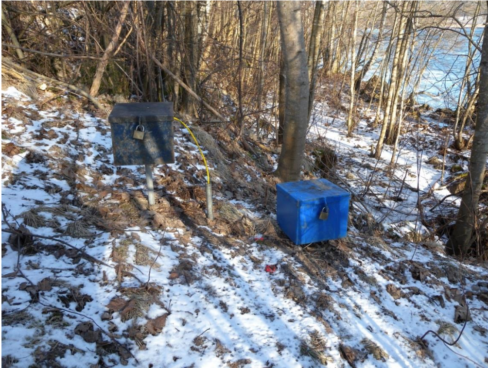
Figure 4-10. Piezometers at the toe of the slope. As can be seen the station is placed some meters from the shore due to the vegetation and the coarse erosion protection material placed next to the river.
