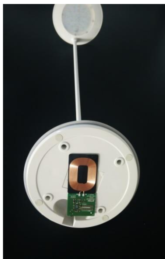
Figure 3.21: A wireless charging receiver mounted underneath the stand.
