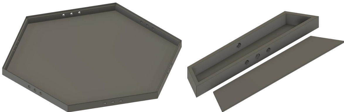
Figure 3.8: Models of charging module (left) and power supply module (right) created for 3D printing. The two modules are not to scale – compare to Figure 3.7.
