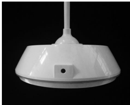
Figure 3.20: The hole left by the lamp's DC power jack.
