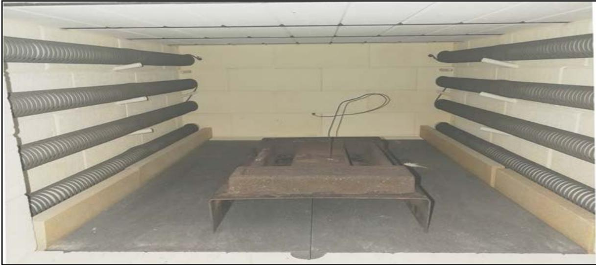
Figure 4.3. Oven 10 is used for the practical heat treatment experiments. The stress lattice is shown in the middle and a thermocouple is put inside the lattice through a drilled hole. Note the shadow of the thermocouple at the back of the oven.
