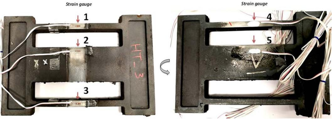
Figure 4.6. The location of strain gauges at the heat treated stress lattice. The two gauges to the right have already been coated in order to prevent them being damaged.
