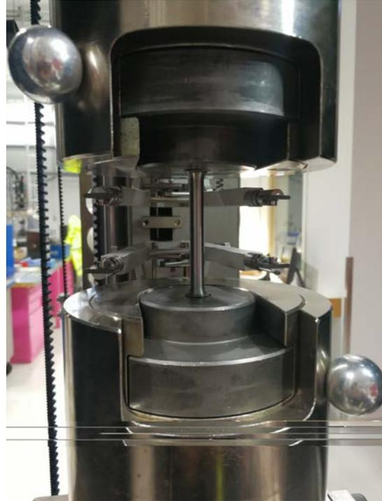
*Zwick 1486 Machine used for tensile testing. The picture to the right is a close up of the tensile test bar.*
