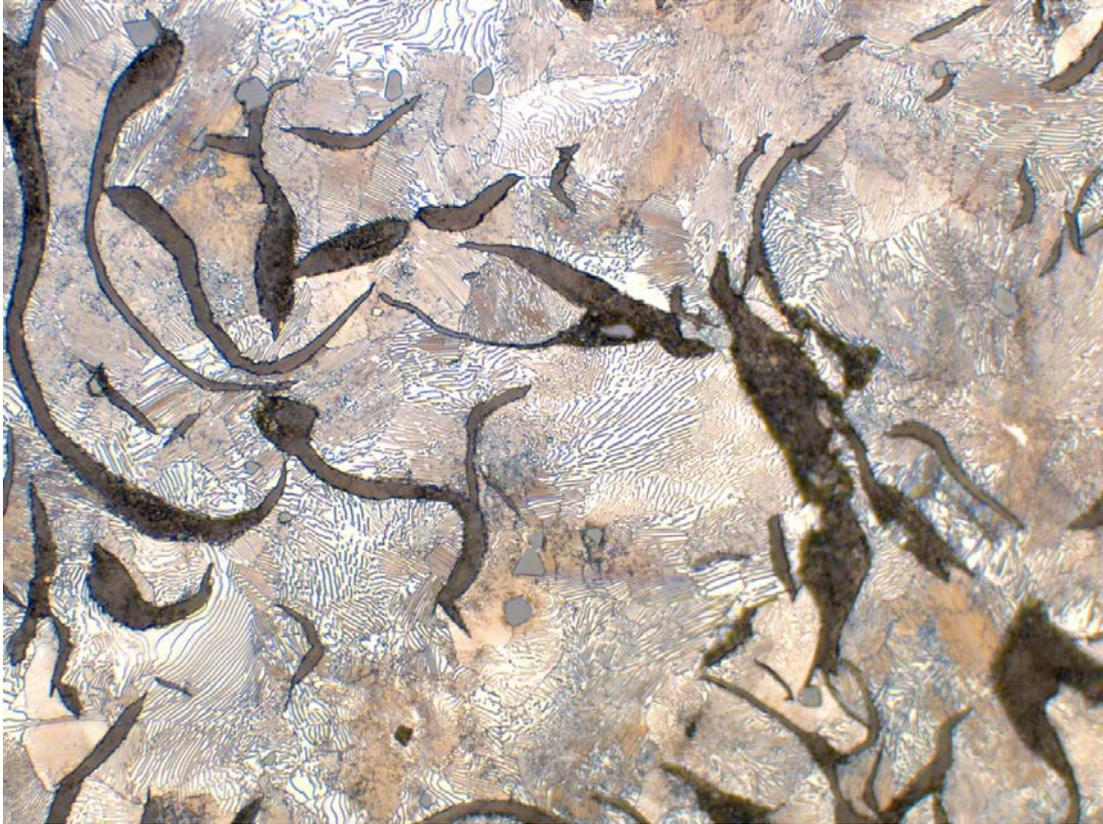
*Microstructure after 650 °C, 5h heat treatment*
