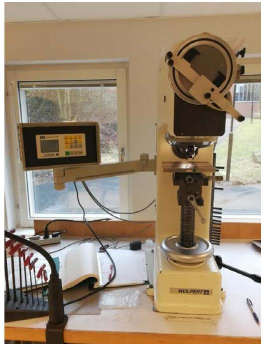
*The heat treatment Oven 10 used for the practical testing and the Brinell hardness machine comp. no. 8900044/0001.*
