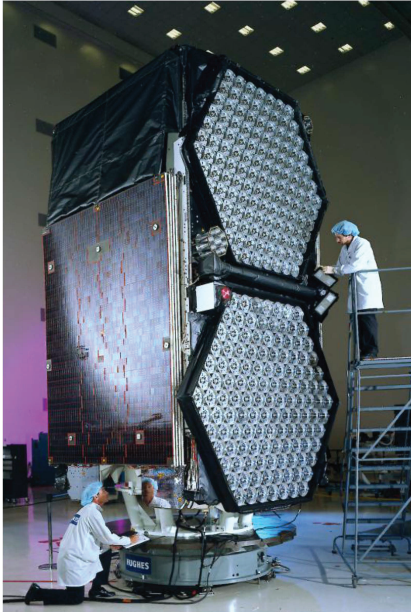
Figure 4.2: Two dense DRA:s of patch-excited antennas for MEO communication at S-band. For GEO applications, an order of a thousands elements is expected.
