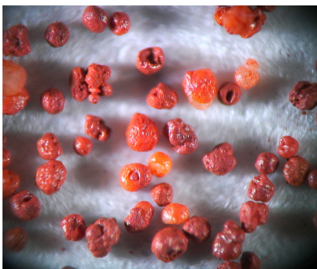
Fe-based, impregnated OC (≈ 100-200 μm)
