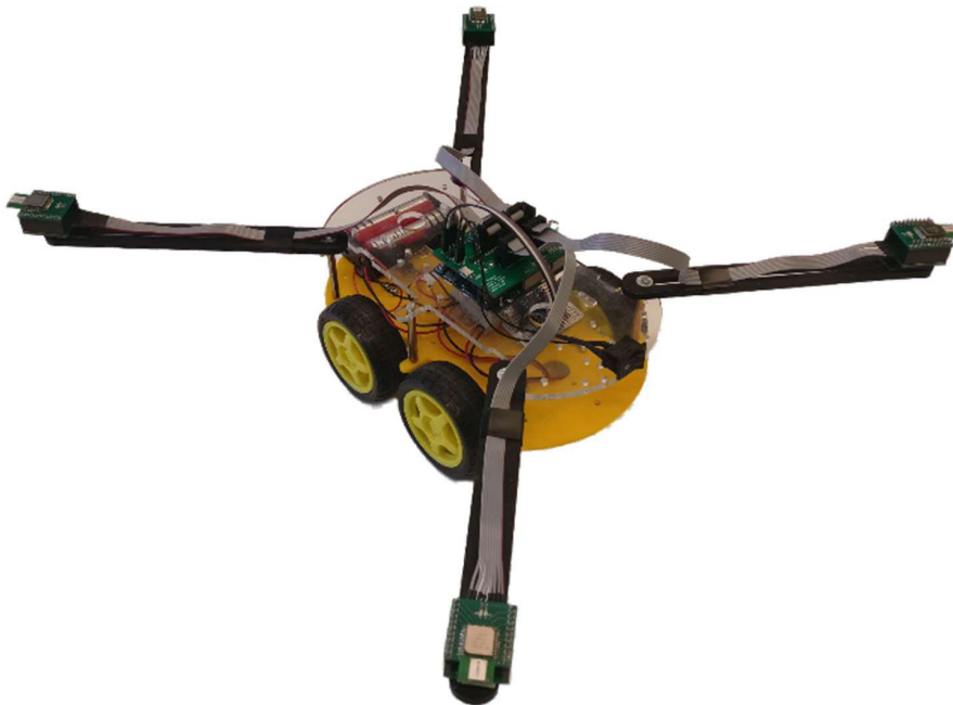
Fig. 4.22. Physical implementation of the system mounted on the 4WD chassis
