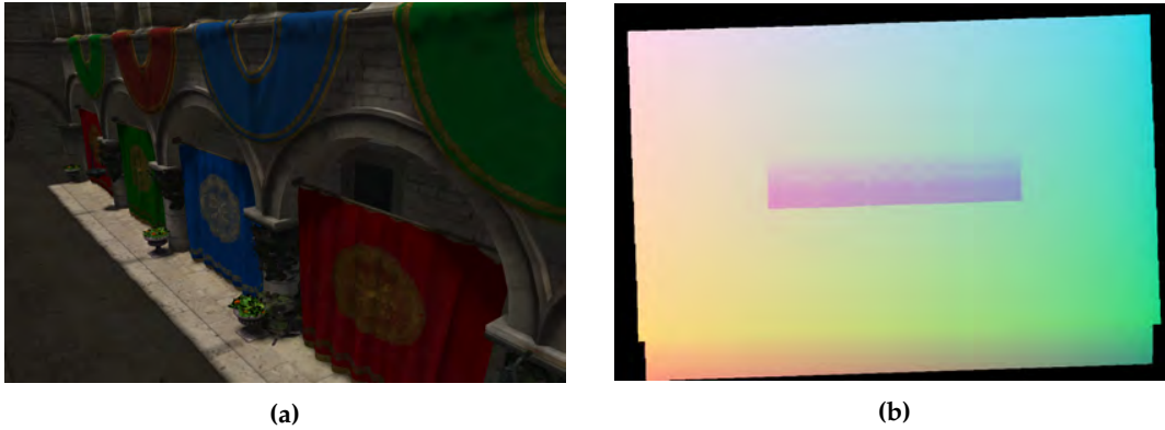
Figure 26: (a) A light source illuminates areas in a scene. (b) Visualization of the RSM of the light source. The (x, y, z) -coordinates stored at every texel are visualized as RGB-values.
