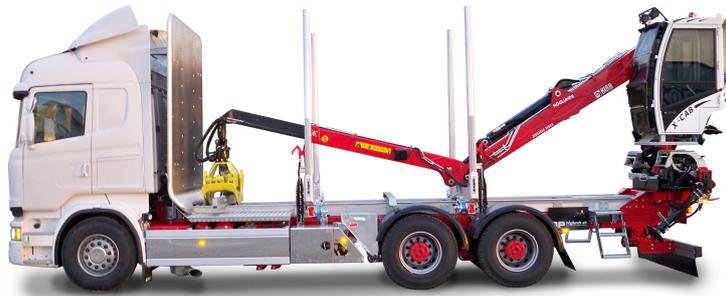
**Figure 1.1:** A logging truck with an arm which can be used to pick up logs.
