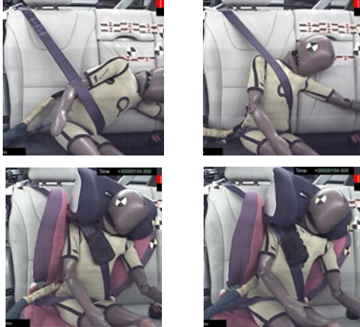
Figure 7. Maximum lateral excursion of the Q6 in side impact; top left: no pretensioner, IBC; top right: pretensioner, IBC; bottom left: pretensioner, booster seat without ISOFIT; bottom right: pretensioner, booster seat with ISOFIT.
