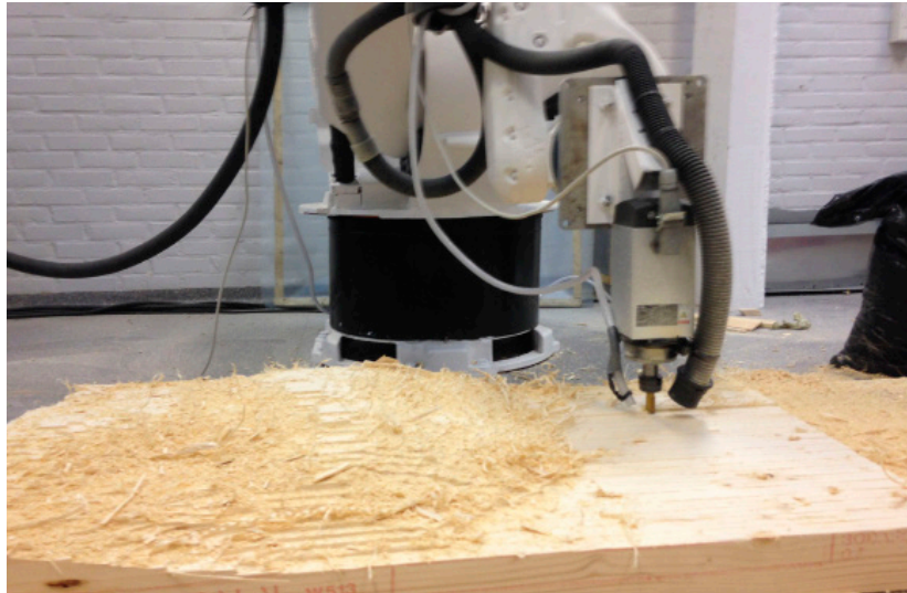
First part of milling process called roughening, using a wide drill bit to get an approximate surface
