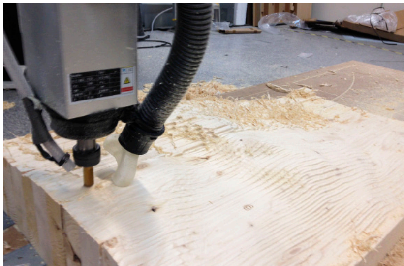
Second program of milling process called surfacing, resulting in a smooth surface
