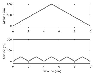
Figure 4.4: Two examples of topographies that has the same GTA-class (PFLAT), but display distinctive characteristics. In the top plot  $L_h = 10$  km, in the bottom one  $L_h = 2$  km.
