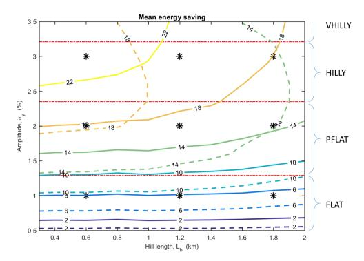
Figure 4.5: Contour plot of the average energy saving ( $\tilde{q}$  in percentage): with solid line showing the m=40 tonne result and a dashed line for m=80 tonne. Additionally, the limiting values of  $\sigma_y$  for the GTA classes is shown in dotted red. Note that the efficiencies of the ICE and battery are different from the corresponding plot in [2].
