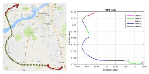
Figure 3.3: Two perspectives of the transport mission in the case-study: the left figure shows the route on a map, while the figure on the right shows the speed limits. Originally published in [3].
