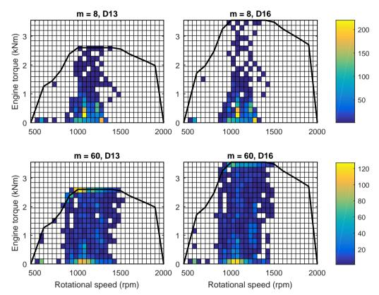
Figure 3.6: Two-dimensional histograms of engine work points, with torque and speed averaged over 1 Hz. The colours show the total operation time (in seconds) in each area: the 10-tonne result in the top row and 56 tonnes in the bottom; left column shows the D13 engine and right shows D16. Note that the colours have been normalized within mission, i.e. the colour indicates the same numbers for equal masses but not equal engines.
