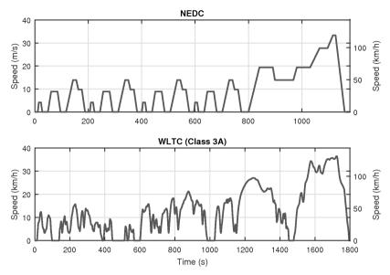
Figure 1.2: Vehicle speed as a function of time for NEDC (top) and WLTC (bottom) [17].
