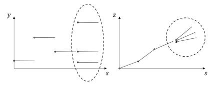
Figure 4.2: The principle of the recursive model. Note that the altitude z corresponds exactly to the topography parameter in the OC-format.
