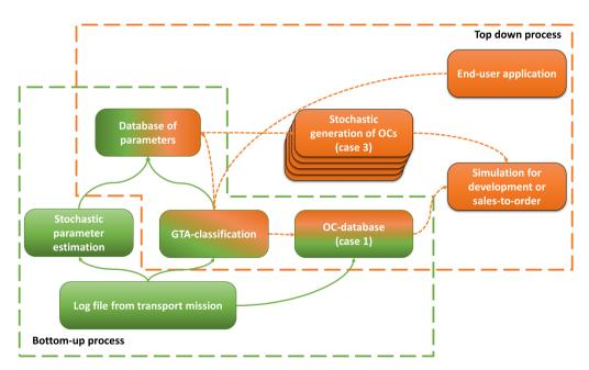
Figure 4.9: Another way of seeing the OCEAN-process than in Fig. 4.1: here the various parts of the thesis are shown explicitly. It is also shown what methods and parts the bottom-up and top-down processes use and create.
