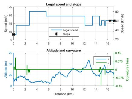
Figure 3.4: Non-trivial parameters of the case-study OC, apart from the speed bump. Top figure shows the speed and stops, bottom figure shows the curvature and topography. Originally published in [3].
