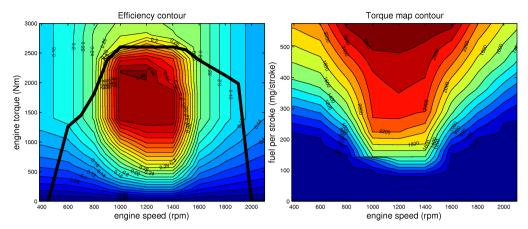
Figure 2.3: Typical efficiency and torque maps (though synthetic) for heavy-duty diesel engines. The left contour shows the engine efficiency  $(P_{out}/P_{in})$  and the right shows the steady-state torque output  $T_e$  in Nm.
