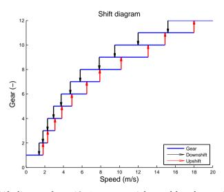
Figure 2.4: Shift diagram for a 12-step, sequential, speed-based gear choice strategy.
