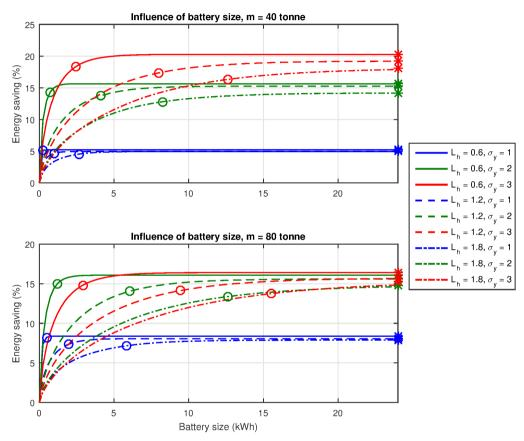
Figure 4.6: Plots of energy saving as a function of battery size, for the nine road combinations. Note that the efficiencies of the ICE and battery are different from the corresponding plot in [2].
