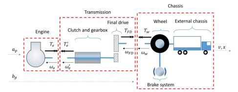
Figure 2.2: A stylised high-level free body diagram of the different subsystems involved in the longitudinal dynamics.
