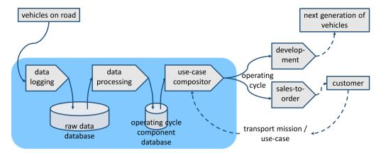
Figure 4.1: A development process that shows how to choose appropriate OCs based on user application. See also Fig. 4.9.
