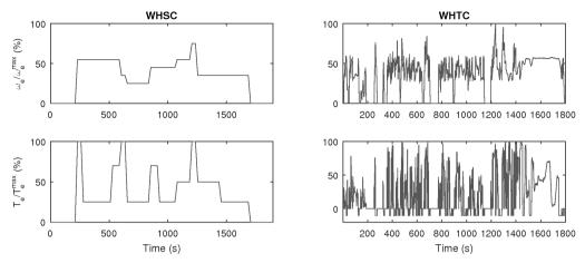
Figure 1.3: The engine load cycles WHSC (left) and WHTC (right). Top row shows percentage of maximum engine rotational speed  $(\omega_e/\omega_e^{\max})$  and the bottom row shows percentage of maximum engine torque  $(T_e/T_e^{\max})$ , both as functions of time.
