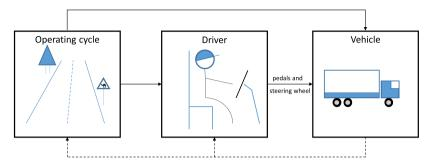
Figure 2.1: The principles of a modular forward simulation with individual models for the mission (operating cycle), the driver and the vehicle. Arrows show signal flow.
