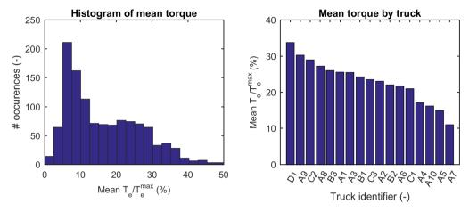
Figure 5.1: Data of the mean torque ratio for the vehicles in the log file. The histogram on the left show how many of the logs have a certain mean torque ratio. The bar chart on the right show what the mean torque ratio is for each vehicle.
