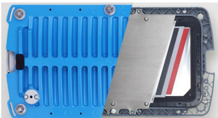
Figure 7. Schematic overview of NiMH battery module illustrating the bipolar stack design [6]. The illustrated components (left to right) are casing, terminal, current collector, anode, separator, cathode, separator, inner and outer stack frame.
