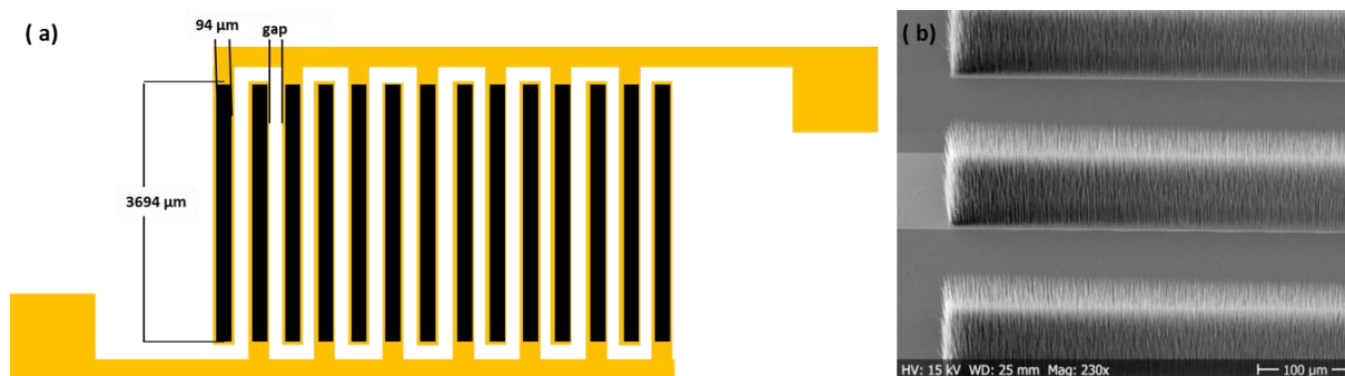
Figure 35: a) Schematic diagram of interdigitated pattern b) CNFs on the digits.
