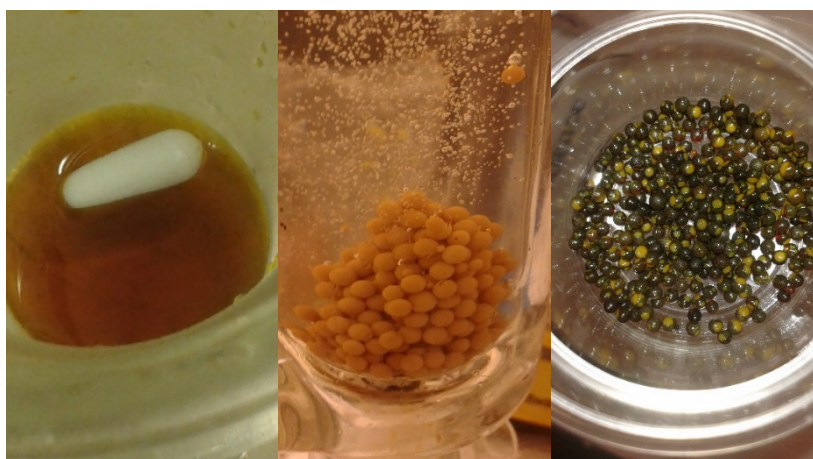
Figure 10. A photo of a gelation process of microspheres containing uranium and glucose, which were made of 1M \text{UO}_2^{2+} . Sol on a cooling bath (left), gelation in hot silicon oil (middle), air dried product (right).
