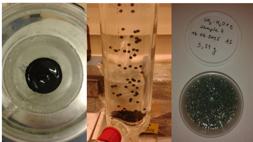
Figure 9. A photo of a gelation process of microspheres containing uranium and carbon nano powder, which were made of a 2M \text{UO}_2^{2+} . Sol on a cooling bath (left), gelation in hot silicon oil (middle), and air dried product (right).
