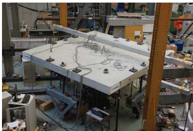
Figure 11. Punching test of an RC slab supported on a column in the centre, loaded at 8 points close to the perimeter (Einpaul, 2016).
