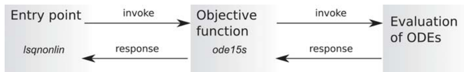
Figure 13: A flow-chart describing the sequence of function invocations in the computational model.
