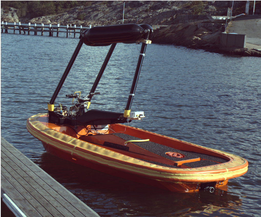
Figure 7.5: The prototype boat that was used instead of a RescueRunner. It is designed to carry more people than the RescueRunner and is therefore slightly larger (4 m LOA as opposed to 3.6 m). Behind the driver's seat is a box holding the Arduino Due, sensors and radio transceiver. An extensions cable connects the box to the antenna mounted in the superstructure above. Another cable connects it to the box mounted below the driver's seat. This is the system developed in [24] which converts the controller outputs to physical movements.
