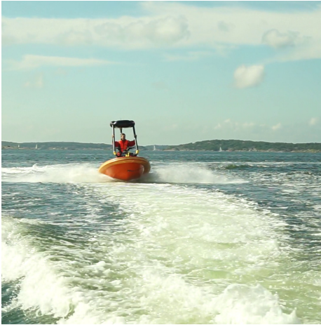
(k) 287 seconds into the test. The RescueRunner cleared the waves without problems and has returned to the desired position behind the lead boat.
