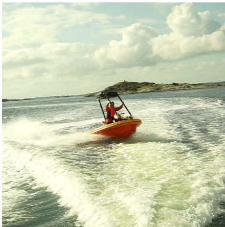
(o) 132 seconds into the test. The RescueRunner experiences oscillations back and forth from which the system does not recover. The test is stopped for further tuning soon afterwards.
