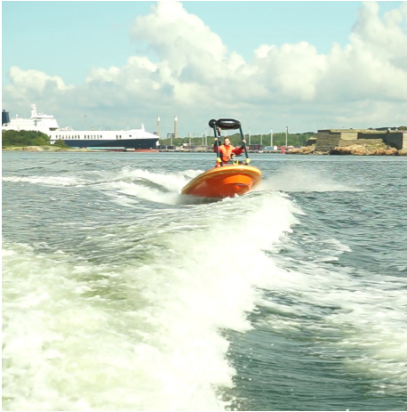
(g) 240 seconds into the test. The control system is less aggressive which makes the RescueRunner take wider turns, but it does not become unstable. The wider turns are compensated by the RescueRunner following behind at a greater distance.
