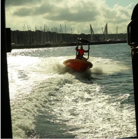
(i) 87 seconds into the test. The RescueRunner starts to fall behind as it struggles to make it over the wave formed by the lead boat's wake.
