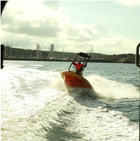
(k) 95 seconds into the test. At the third attempt the RescueRunner clears the wave and subsequently stabilizes behind the lead boat as before.
