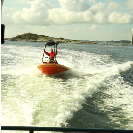
(m) 128 seconds into the test. After successfully completing another turn the RescueRunner makes an unexpectedly hard starboard correction. 7.8n shows that at this time the estimated orientation does not seem to match the actual one.
