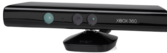
Figure 2.1: The image shows the stand alone Kinect for XBox 360. The apertures on the front from left to right are the IR grid projector, the IR camera, and the RGB camera.
