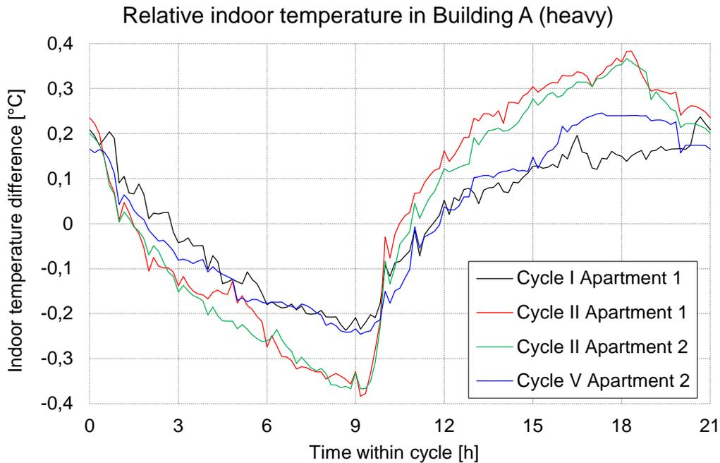
**Figure 4.4** Indoor temperature variations caused by the pilot test. Each curve is based on average values over a period of 4–6 weeks.
