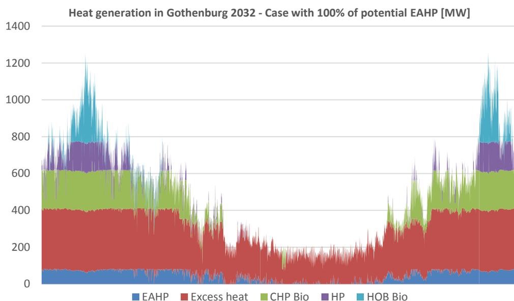
**Figure 5.4** Heat generation in Gothenburg 2032 with EAHP prioritized for base load. 100% of renovated and newly constructed multi-family residential buildings have EAHP. Based on data from (Holm and Ottosson, 2016).
