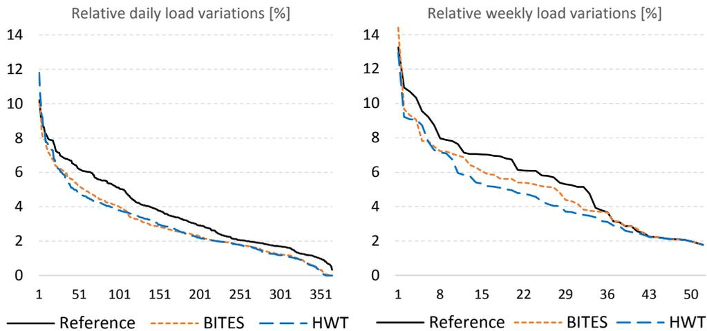
**Figure 4.12** The a) relative daily heat load variations and b) relative weekly heat load variations for the reference, BITES, and HWT, in descending order
