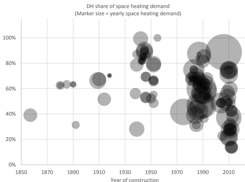
**Figure 5.1** DH share of space heating demand in buildings with DH and EAHP (SPF = 3), assuming all domestic hot water is provided by DH. Markers are transparent, and darker color indicates higher concentration of properties.
