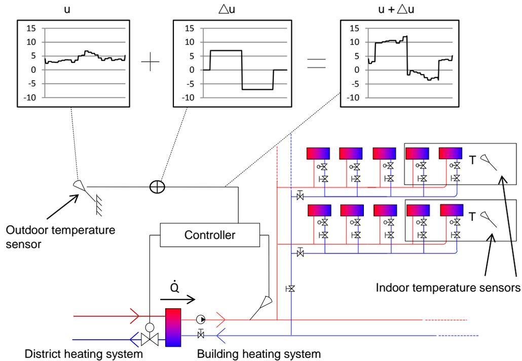
**Figure 4.1** Schematic of how the control was implemented in the pilot test
