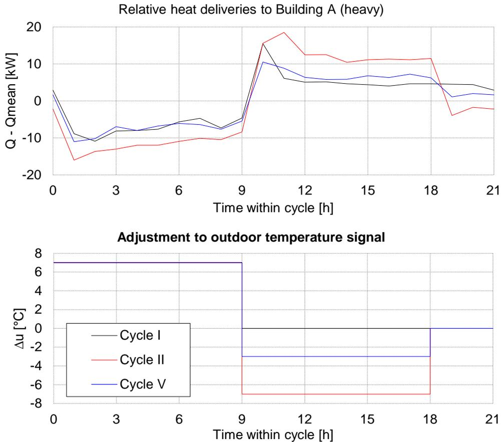
**Figure 4.3** Heat use profiles relative to the control cycle average for Building A. Each profile is based on 5–8 weeks of measurements.
