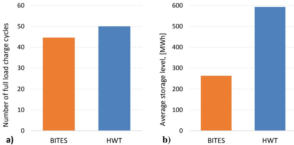
**Figure 4.10** The number of a) full load charge cycles and b) the average energy level in the HWT and the BITES over the year
