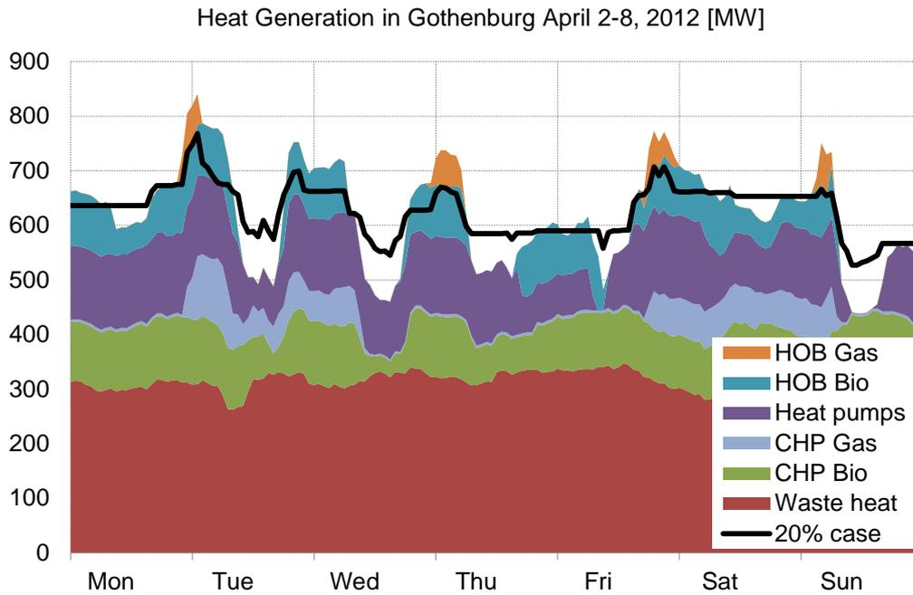
**Figure 4.8** Example of the heat generation in Gothenburg during one week with a possible load curve from the 20% case as an overlay.
