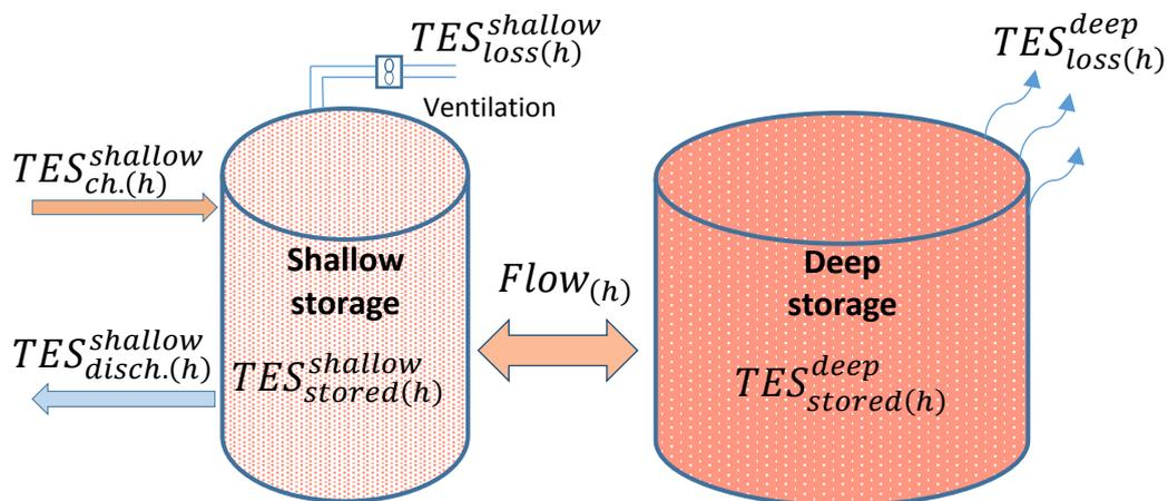
**Figure 4.5** Schematic representation of dynamic model for BITES
