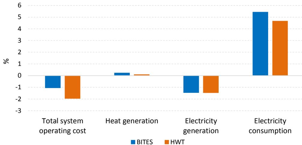
**Figure 4.13** The total system cost, the total heat and electricity generation, and the total electricity use for the cases with the BITES and the HWT, as obtained from the modeling and compared in percentages to the reference case with no TES
