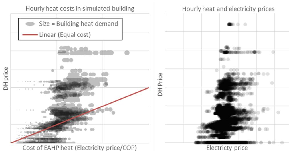
**Figure 5.3** Left figure: Comparison of heat cost from the two heat sources where the COP of the EAHP is considered every hour, 2013–2014. Points below the line indicate that heat from DH is cheaper than heat from the EAHP. Right figure: Figure 3.3, scatter plot of hourly heat and electricity prices 2013–2014.
