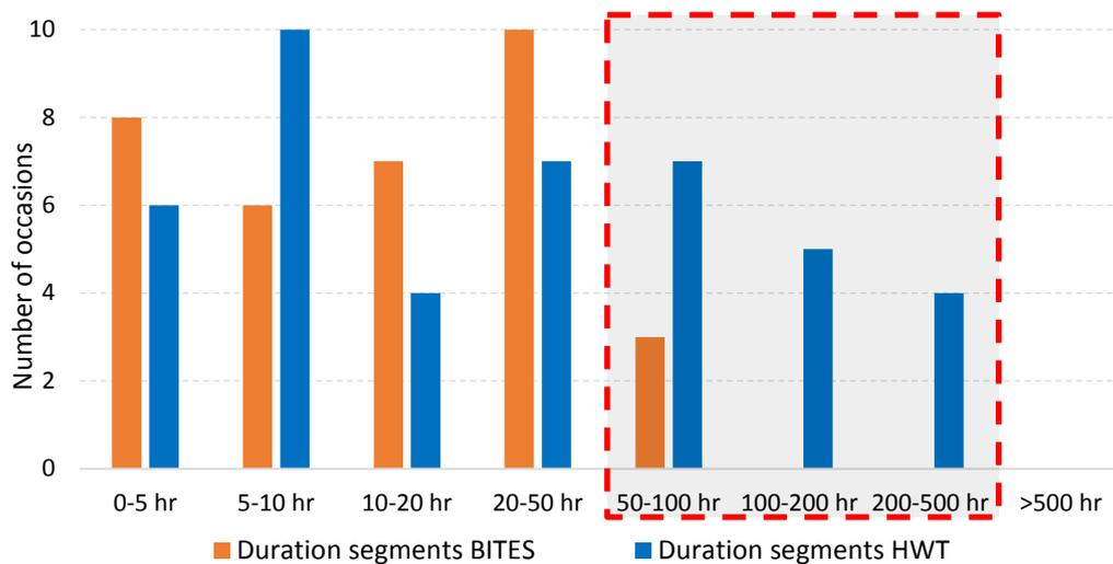
**Figure 4.11** The number of occasions classified in duration segments when the HWT and the BITES remained charged at a level higher than 1,000 MWh, as obtained from the modeling
