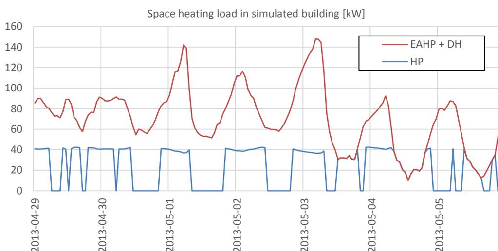
**Figure 5.2** Operation of the base case heating system with shifting load priority during one spring week (warm days and cold nights)
