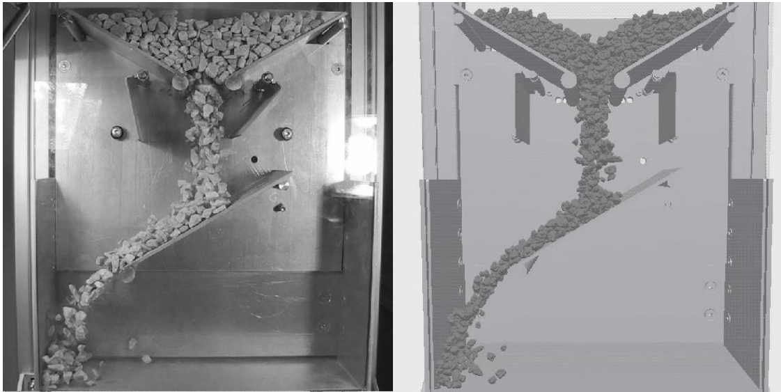
Figure 33. The left hand side image shows a frame from a recording of a real experiment after the first stream of particles has travelled through the device. The right hand side image shows the corresponding flow in the simulation environment.
