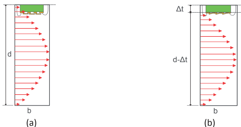
Figure 3-9. E-field contribution with an electrically tunable wall inside the cavity. (a) RF-MEMSs in open state. (b) RF-MEMSs in a closed state.
