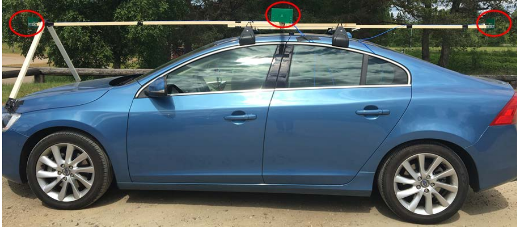
Figure 5.2. Reference module mounted on the vehicle. The red circles show the placement of the antennas.
