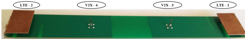
Figure 4.4. Manufactured prototype of the antenna module
