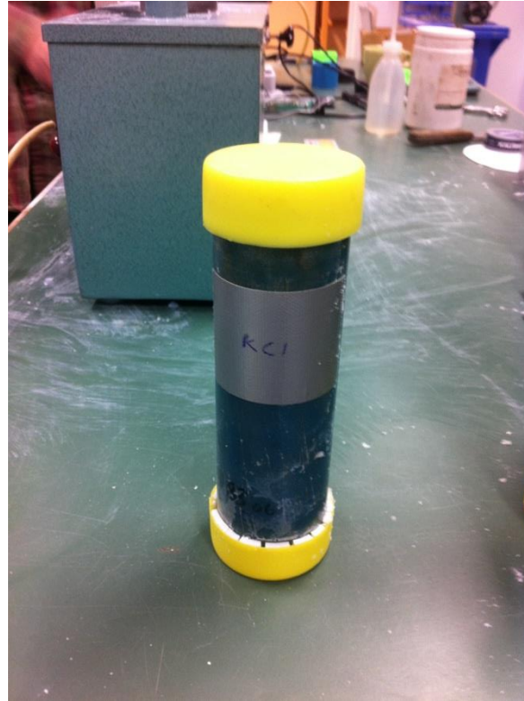
Figure 7 – Cylindrical container used to mould and store the silica sol samples for the uniaxial compression test.
