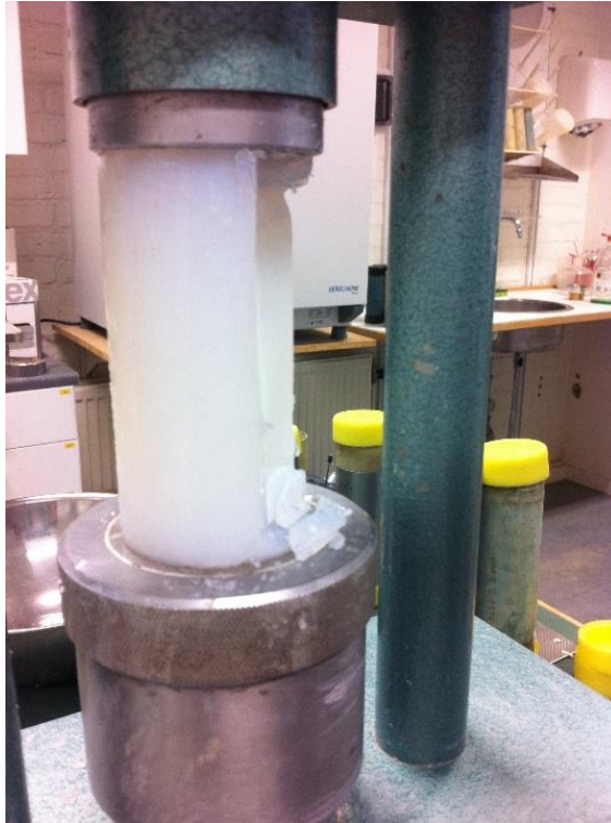
Figure 13 – Vertical fracture plane consistent with the results of Butrón, Axelsson and Gustafson (2007).
