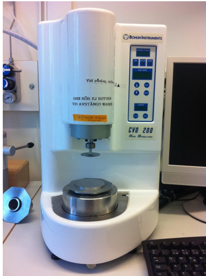
Figure 9 – Rheometer with oscillating plate setup.
