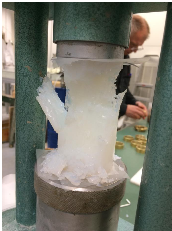
Figure 14 – Cone-shaped fracture of the specimen after using membranes during a uniaxial compression test (Photo taken by Emilia Funehag).
