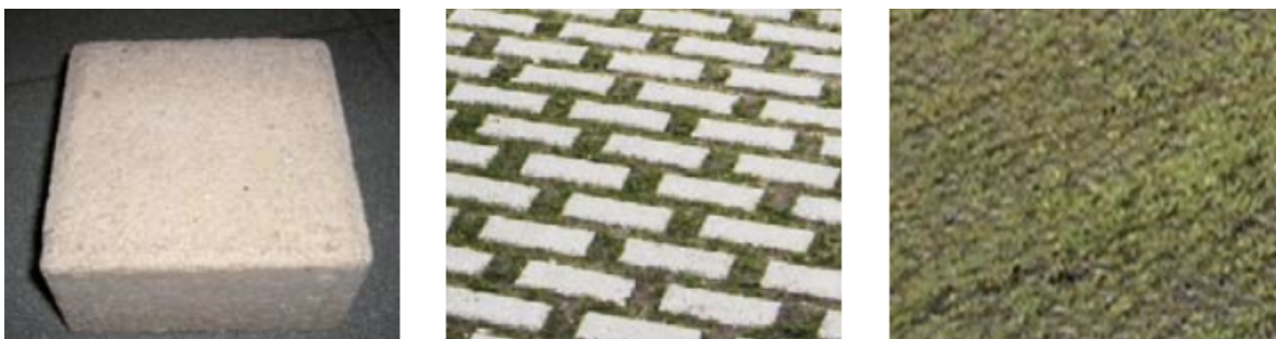
Figure 3.10: Different types of porous pavements: porous concrete; concrete paving with drainage openings; turf paving. (Luchesi, 2008b)
