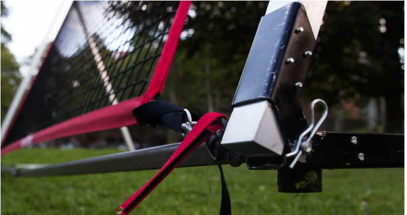
Figure 6.17 Front feet and rotation mechanism
