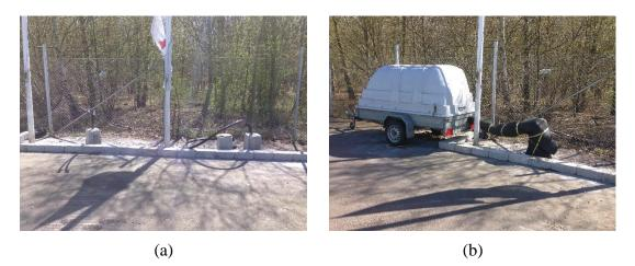
Figure 3.2 HP-Borrningar testing facility: (a) Driven precast pile heat exchangers (b) Thermal response test being performed on a driven concrete pile heat exchanger.
