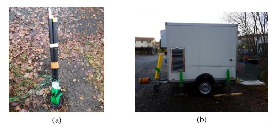
**Figure 3.1** Chalmers testing facility: (a) Driven steel pile heat exchanger (b) Thermal response test being performed on the driven steel pile heat exchanger.
