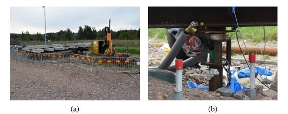
**Figure 3.3** NCC recycling facility: (a) Driven pile heat exchangers with mechanical loading (b) Mechanically loaded and fully instrumented steel pile exchanger with observation holes.
