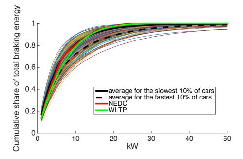
Figure 12: For the assumed midsize car (m = 1500 kg,  $C_D^*A = 0.7 m^2$ ) and for each movement pattern, the cumulative likelihood that the braking power is less than a given power level. Rolling resistance coefficient  $c_r = 0.01$ .
