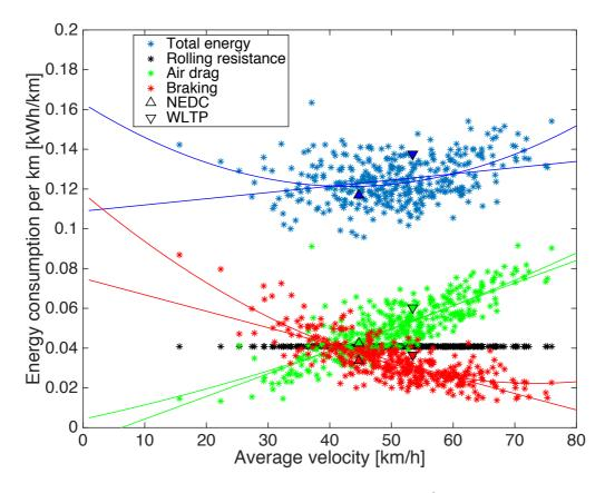
Figure 11: For the assumed midsize car (m = 1500 kg,  $C_D^*A = 0.7 \text{ m}^2$ ), for each movement pattern (asterisks: individual vehicles in our data; triangles: test cycle values, see legend), the average energy at the wheels (components: rolling resistance, air drag, and braking) lost per km of driving and its components, as a function of the average velocity. Solid lines correspond to linear and quadratic regressions. Rolling resistance coefficient  $c_r = 0.01$ .
