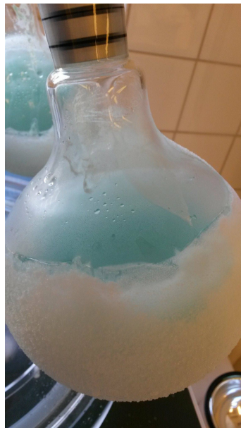
Figure A.2: visual presentation of the freeze drying step of the catalyst
