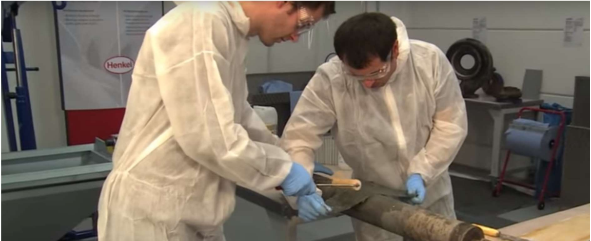
Figure 22 The wrap is wound around the pipe (Youtube Woronko premium partner Loctite partner channel, 2014).
