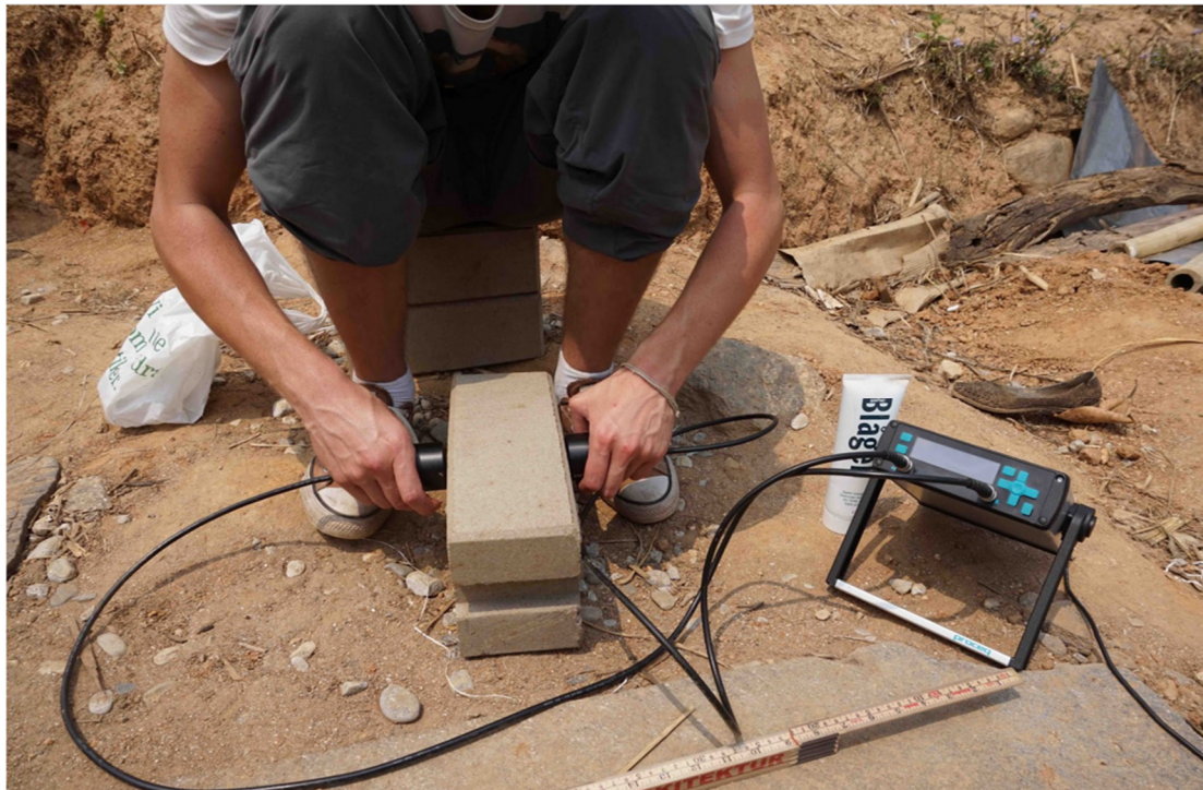
Figure 27. Ultrasonic Pulse velocity test with a Pundit lab and two 54 kHz transducers in Majhi Gaun.
