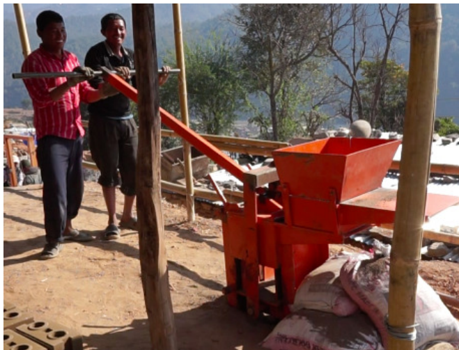
Figure 10. CSEB machine used in Majhi Gaun.
