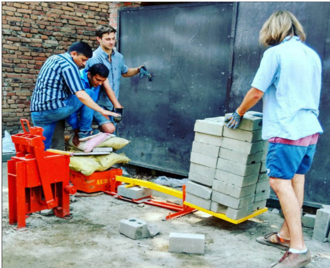
Figure 28. Test of CSEB with 250 kg on the loading plate.
