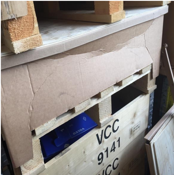
Figure 25: A One Way box that has collapsed. The reason why can be that the boxes that are stacked on top of it are carry too much weight.
