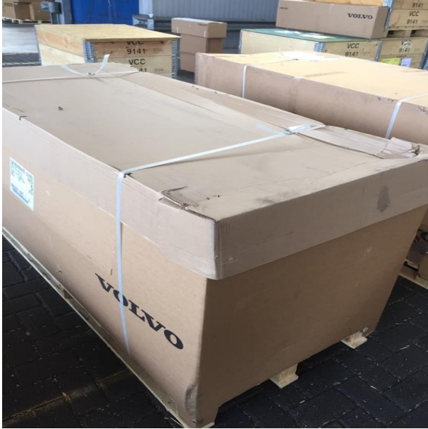
Figure 24: The One way packaging is collapsed due to the tensioned rope.
